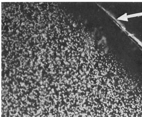
Fig. 1. Void morphology in nitrogen-gasified PC. Heat treatment 160°C, 30 min, 1500 psi N 2 , cooled to room temperature, followed by 150°C, 15 min, 1 atm. Magnification 30X. Arrow indicates surface of specimen.
